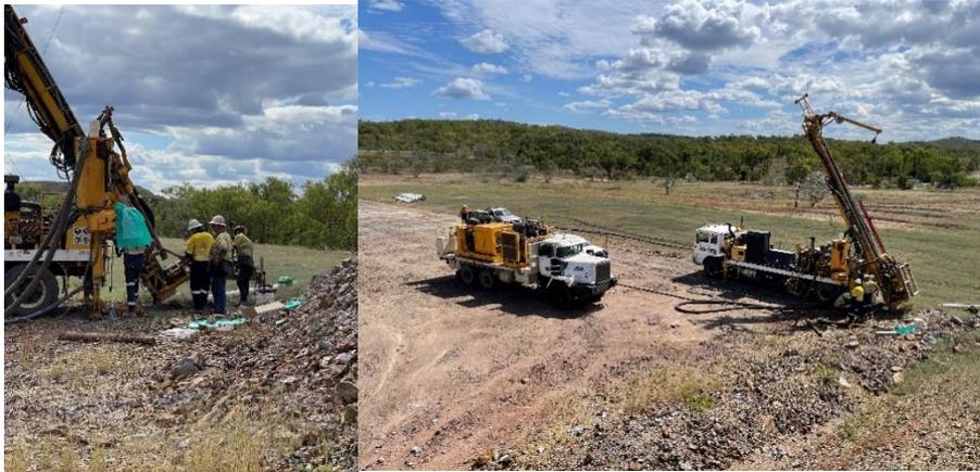
Figure 2 – Drill rig setting up on the rehabilitated portion of the open pit.
